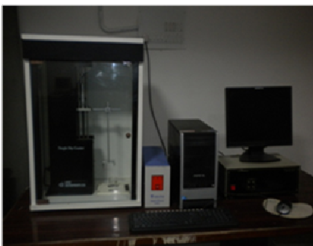
Single Dip Coating system
